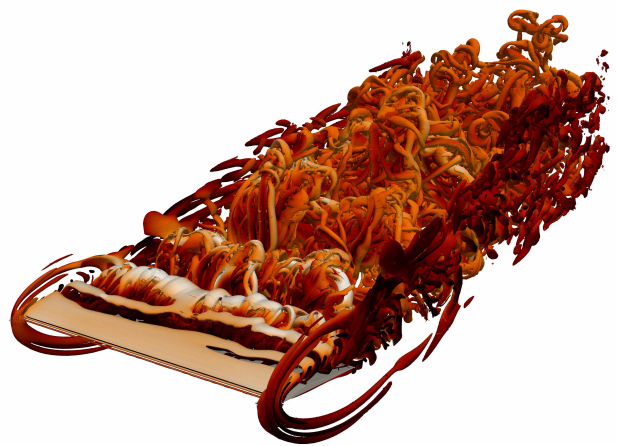
Figure 10: Instantaneous snapshot of a Q-criteria iso-surface coloured by velocity magnitude around a triangular aerofoil for a Martian helicopter obtained using the compressible Navier–Stokes solver in PyFR. Image is from Fig. 10 of Caros et. al [64]. Copyright Caros et al. Reused with permission.
